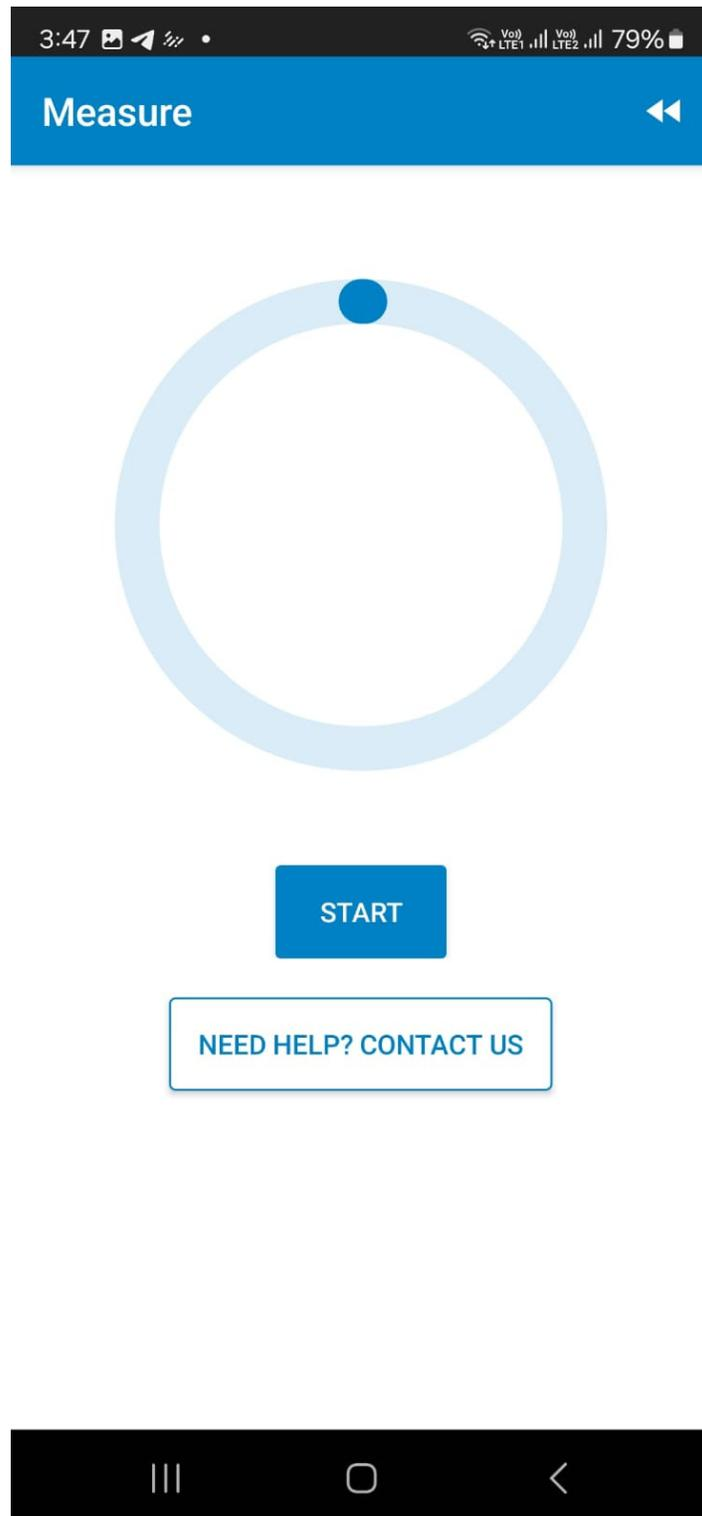
Pound on the surface with your closed fist to instigate the resonance until the measurements are complete.
