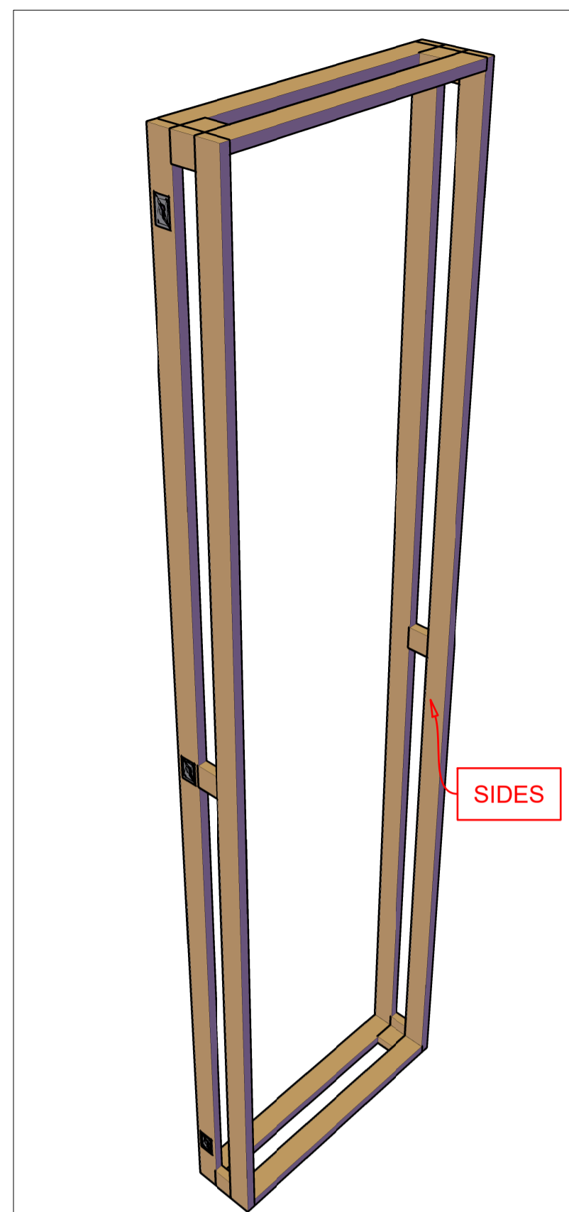
1. ASSEMBLE TOP, BOTTOM, AND SIDES USING DOWELS AND GLUE. MAKE SURE THE UNIT IS 'SQUARE' (90 DEGREE CORNERS).
