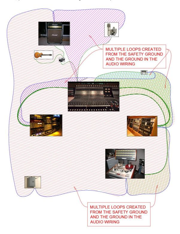
Loop area will introduce the ambient electromagnetic field into the audio system; 50 or 60 Hz depending on your local power frequency plus all the unwanted harmonics and electromagnetic hash that may be present due to dimmers and other hash producing equipment, etc. The solution is to collapse the loop.
