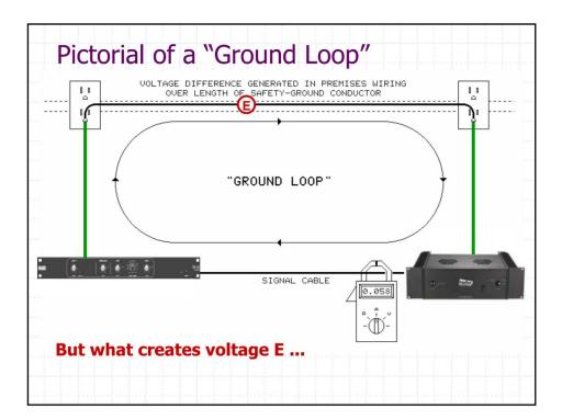
"Broadly, the purpose of grounding is to electrically interconnect conductive objects, such as equipment, in order to minimize voltage differences between them. An
