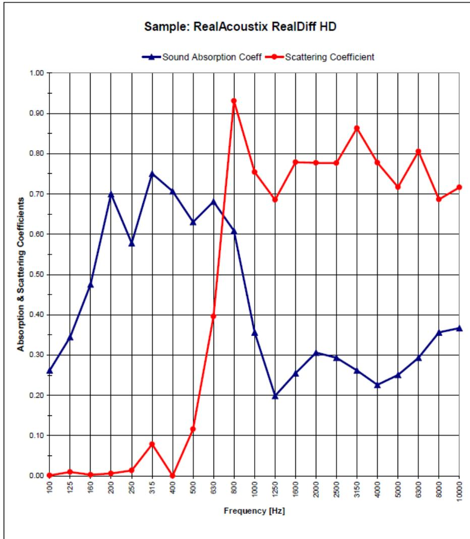
The blue line represents absorption and the red line is supposed to be diffusion. These types of results could be deemed to be reasonable under most conditions as it lives within the expected confines assumed by most to be accurate. It might be so if there were some way to define the nature of the waveforms, which there is not.
