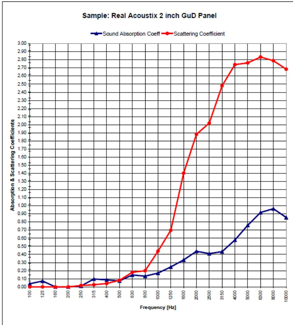
Note that the results, the coefficients, exceed 2.80 in the diffusive range. This test was conducted (7) times to ensure the results. This would indicate that the panel actually amplifies the signal, which is beyond believable, of course. While this is certainly a worst-case scenario, it is all-together too common and shows the Achilles heel of the -1 standard as well as coefficients in general.
