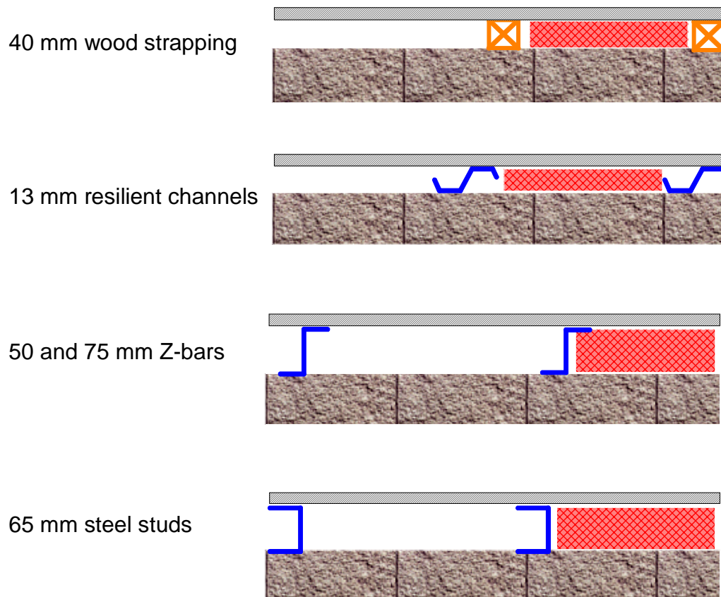
Figure 2: Techniques used to attach drywall to the block walls. In each case the walls were tested with and without glass fibre in the cavity.
