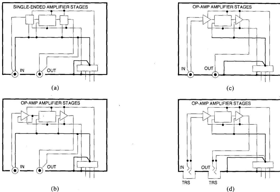
Fig. 7. Unbalanced devices. (a) Older device; I/O connector pin 1s connected to audio signal ground. (b) Modern device with unity-gain noninverting input; I/O connector pin 1s connected to audio signal ground. (c) Device with differential input referenced to device chassis; I/O connector pin 1s connected to chassis ground. (d) Device with differential input "forward referenced" to source device; I/O connector pin 1s connected to chassis ground.
