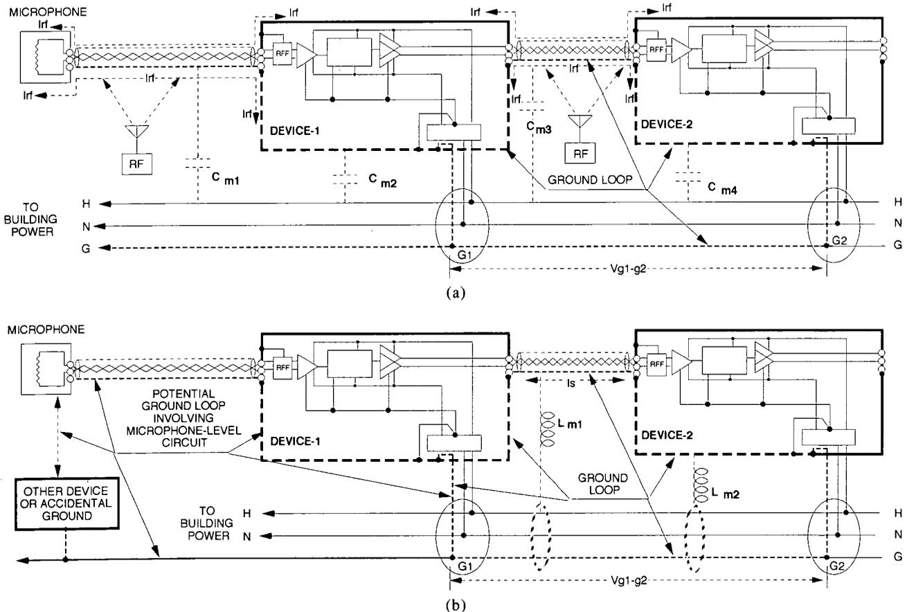
Fig. 5. Noise current flow into generic ASP system. (a) Due to electric and RF field coupling. (b) Due to magnetic-field coupling into ground loops.
