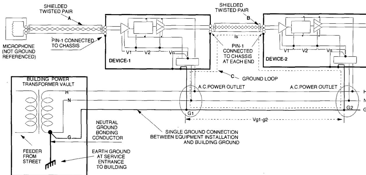
Fig. 4. Schematic diagram of generic ASP system showing interconnections between equipment and building power and ground.
