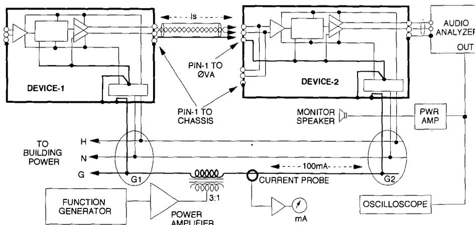
Fig. 8. Pin 1 problem demonstration test setup.
