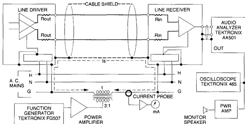
Fig. 2. Test setup used to measure shield-current-induced noise (SCIN).
