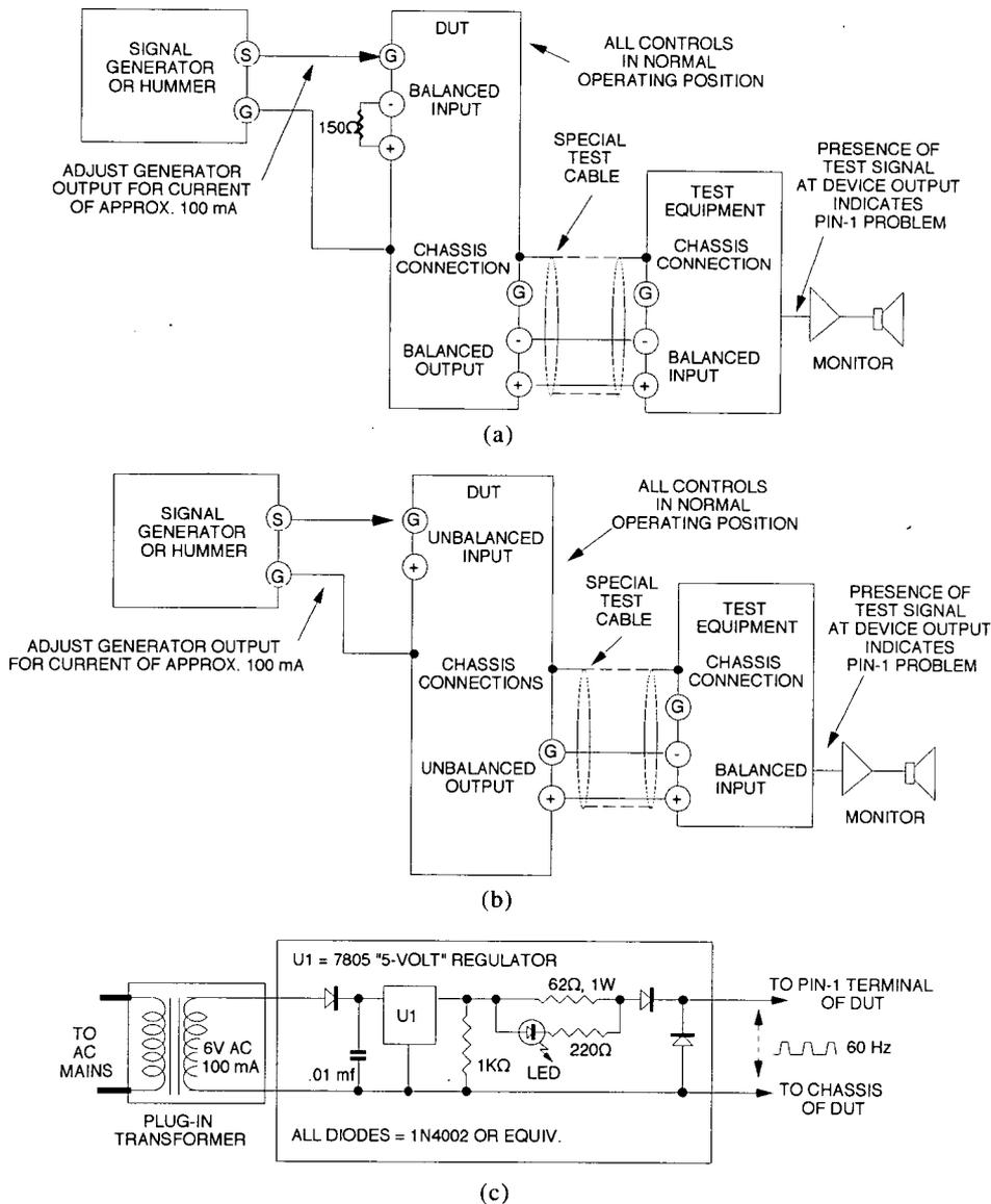
Fig. 10. (a) Connections to balanced device under test (DUT). (b) Connections to unbalanced DUT. (c) "Hummer 2" pin 1 problem locator [12].
