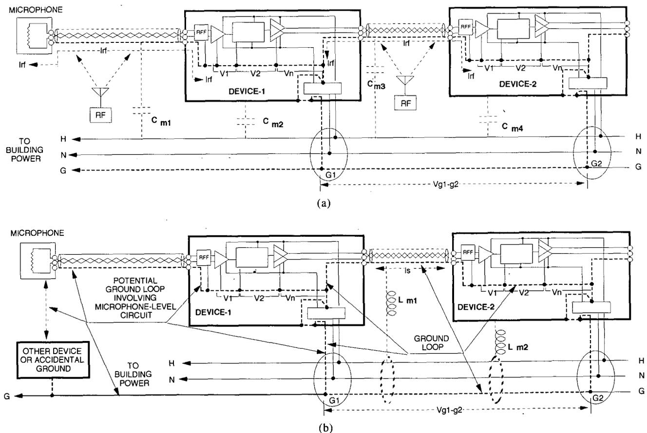
Fig. 6. Noise current flow into generic ASP system with pin 1 problem. (a) Due to electric and RF field coupling. (b) Due to magnetic-field coupling into ground loops.
