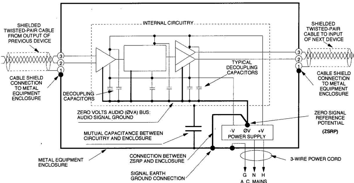
Fig. 1. Generic audio signal processing device.
