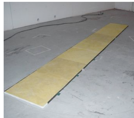
Figure 8: Standard Rectangle sample 9.675 ft (2.95m) L X 7.675 ft (2.34m) W
