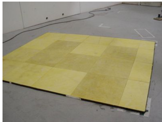
Figure 8: Standard Rectangle sample 9.675 ft (2.95m) L X 7.675 ft (2.34m) W
