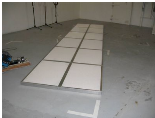
Figure 14: Rectangular Long sample 18 ft (5.49m) L X 4 ft (1.22m) W
