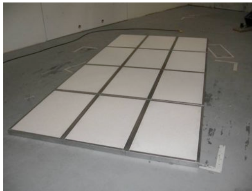
Figure 13: Standard Rectangle sample 12 ft (3.66m) L X 6 ft (1.83m) W
