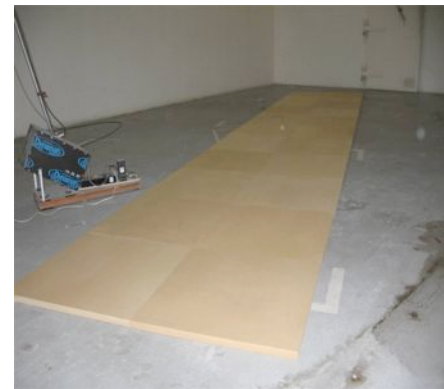
Figure 11: Rectangular Long sample 22 ft (6.71m) L x 4 ft (1.22m) W Material is 1 inch (2.54 cm) thick HDF sealed with Marine Varnish
