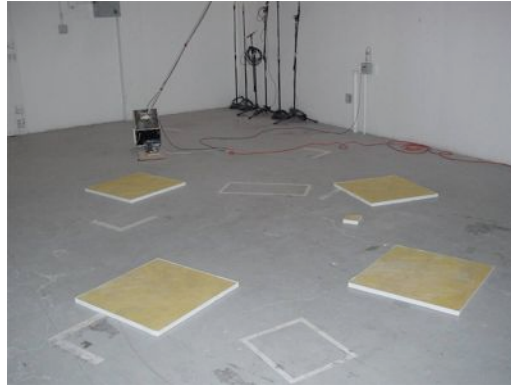
Figure 10: Scattered pieces sample 4 pieces 2 ft (0.61m) X 2 ft (0.61m) 1 piece 0.07 ft (0.02 m) x 0.07 ft (0.02 m)
