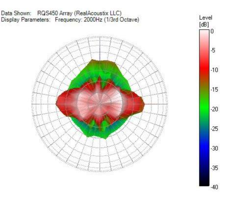
In the Balloon Display view you may select any frequency data set from 25Hz to 20KHz. Some of the lower frequency information will be limited dependent on the size of the specimen. Some of the high frequency information will be less useful due to air absorption. This, however, can be compensated for in the viewer settings. The actual useable frequency response is more along the lines of 250Hz to 10KHz.
