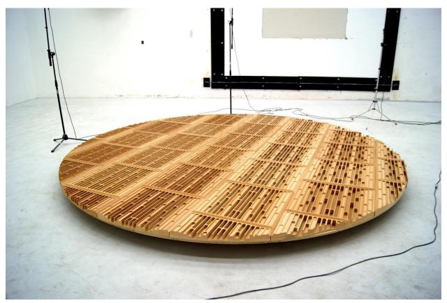
Reverb Chamber set up for ISO 17497-1 Scattering Test
