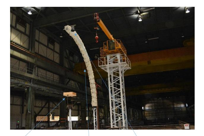
Diffuser under test (19) microphone array Excitation source (speaker)
